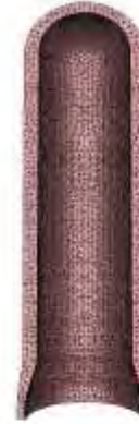
Figure 12 : Mesh of the preform (44 403 nodes, 223 155 elements).
