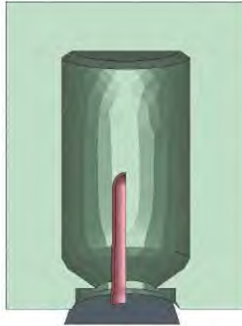
Figure 14 : Geometries of the preform and the mold.
