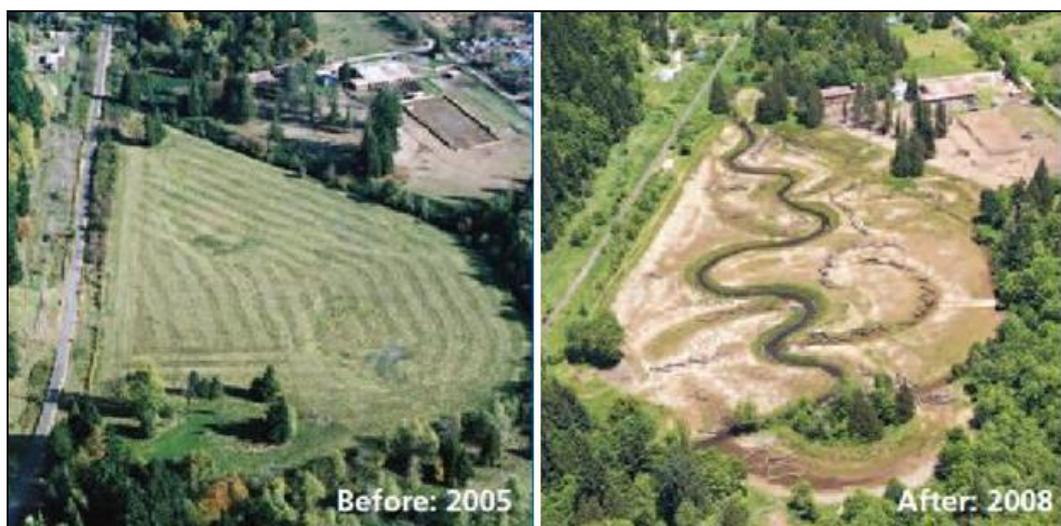
Figure 19 Exemple de re-méandrisation de rivière, Source: [Bluegreencities.ac.uk](http://Bluegreencities.ac.uk)
