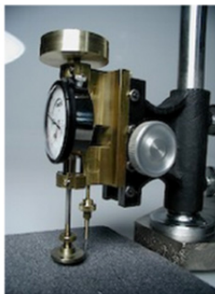
Frazier Schiefer Carpet Thickness Gage (new model with digital indicator is now available)
