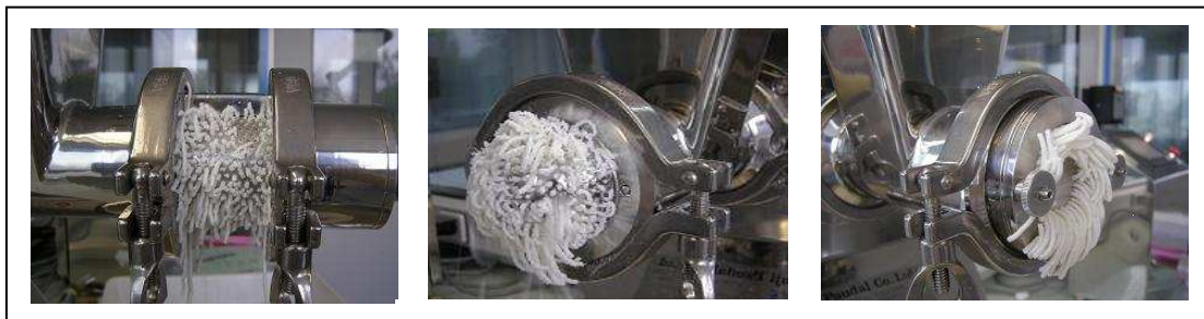
Figure 2- 9: Extrusion of the wet mass for the different extrusion systems: radial, dome, axial.
