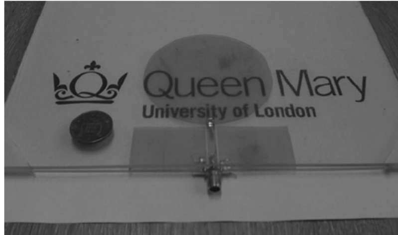
Figure 2-23 Antenne ultra large bande optiquement transparente [21].
