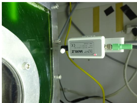
Figure 60 : Photograph of the PAM sensor, used to measure the Chlorophyll a fluorescence at the PBR surface.
