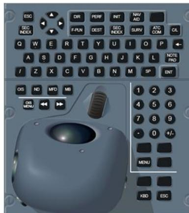
Figure I.4 KCCU (Keyboard Cursor Control Unit)
