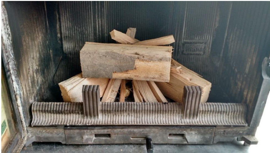
Figure S1: Set-up of the logs in the combustion chamber of the old logwood stove (stove A).
