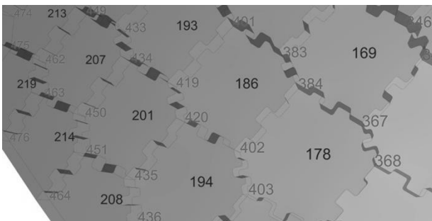
Figure 7: Dovetail detail model – Rendering in Rhinoceros
