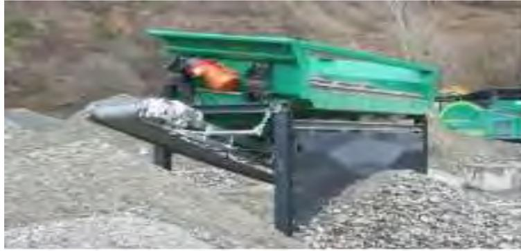
*Figure 9: La machine de criblage*
