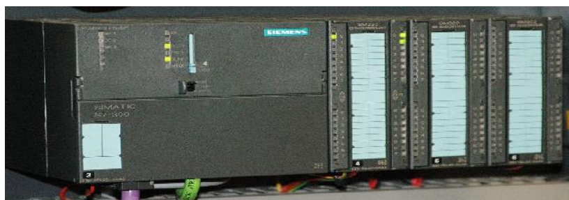
Figure 38: photo Automate Siemens 300
