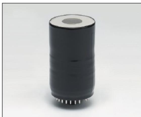
Hamamatsu R943-02 is a 51 mm (2") diameter head-on type photomultiplier tube having GaAs (Cs) photocathode and synthetic silica window. The combination of the GaAs photocathode and the synthetic silica window allows high sensitivity over a wide spectral range from UV to IR (160 nm to 930 nm).
