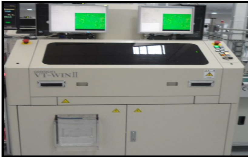
Figure 20: La machine "OMRON VT WIN2" qui effectue le test AOI
