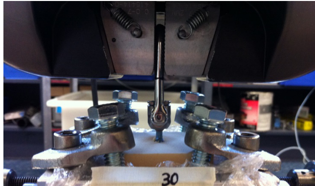
Figure 3. The test fixture placed in the material testing system for pullout test. Custom test fixture was the same as for indentation and torque measurement tests.
