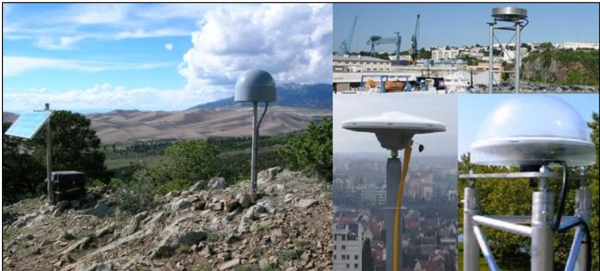
Figure 1 : Station Permanente GNSS
