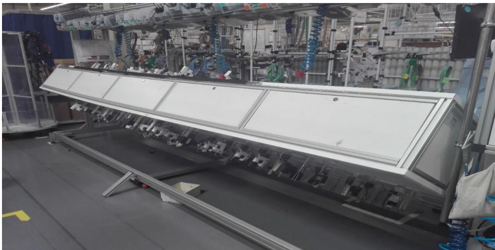
Figure 49: Installation de Clip Checker rotatif
