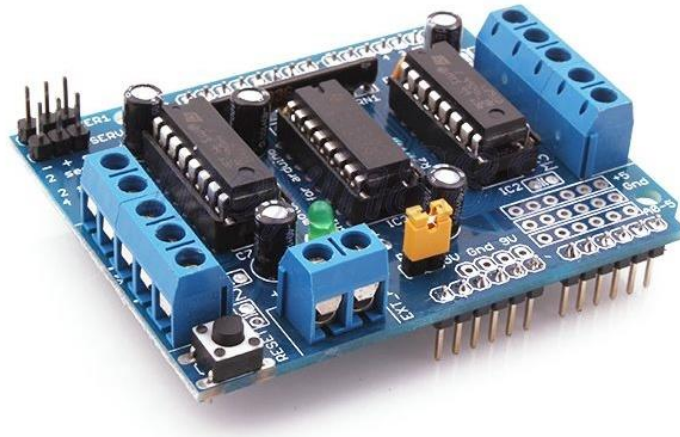
Figure 3.10 : Motor Shield I293d
