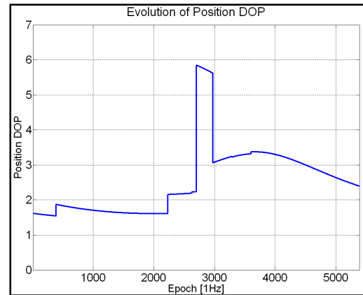
Figure 5.4 Evolution of Position DOP during medium baseline test.
