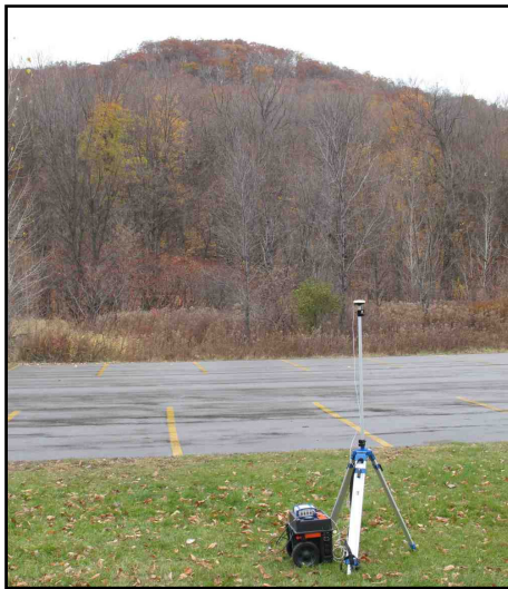
Figure 5.1 Static rover antenna installation for the medium baseline test.
