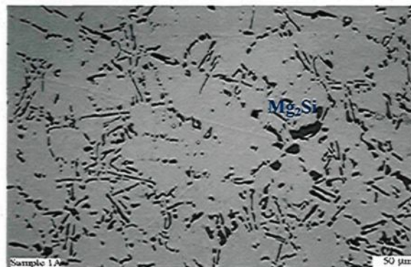
Figure 2.13. Optical micrograph of as-cast Al-7% Si-0.4% Mg alloy. 105
