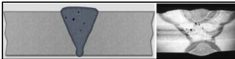
Figure III.20 : Inclusions gazeuses porosités uniformes
