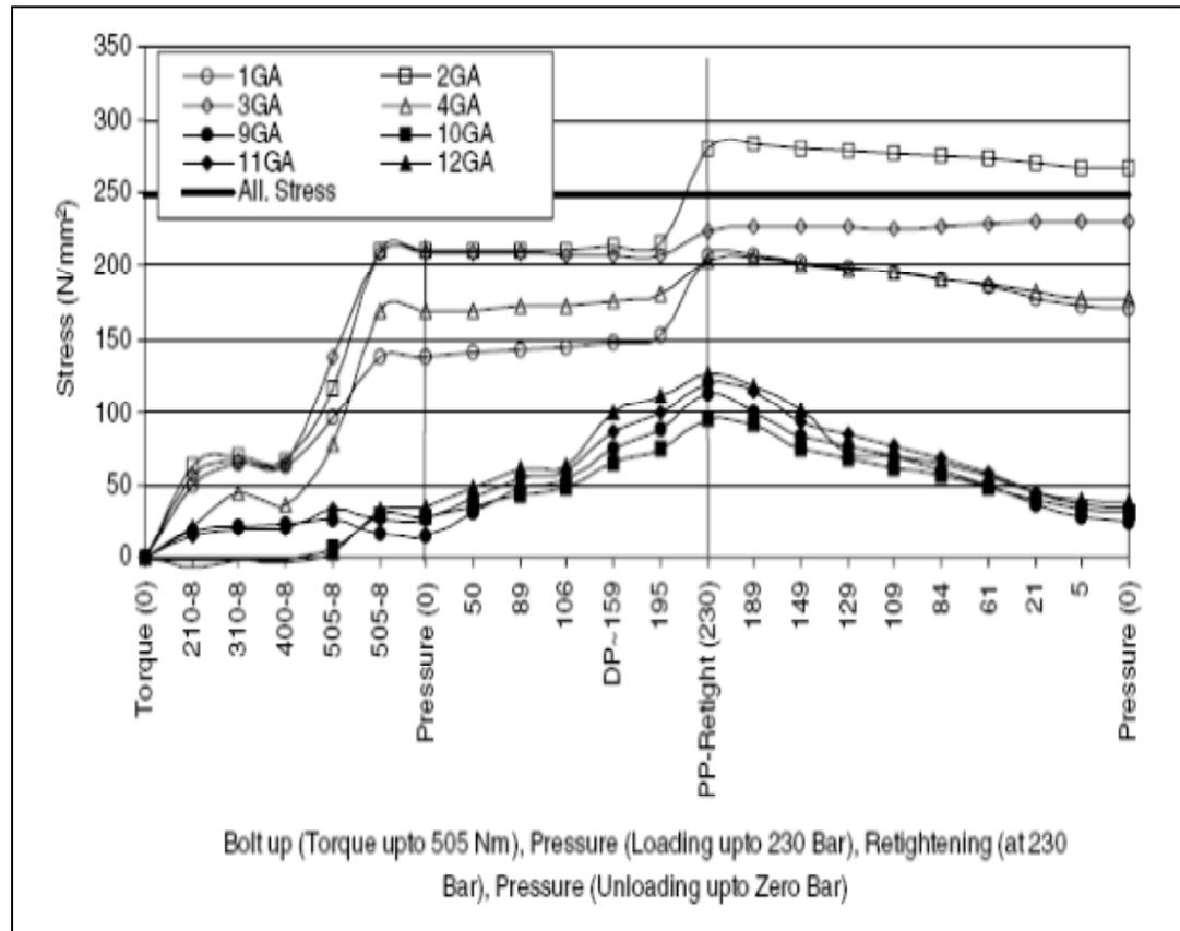
**Figure 2.3 Effect of retightening on maximum principle stress [13]**
