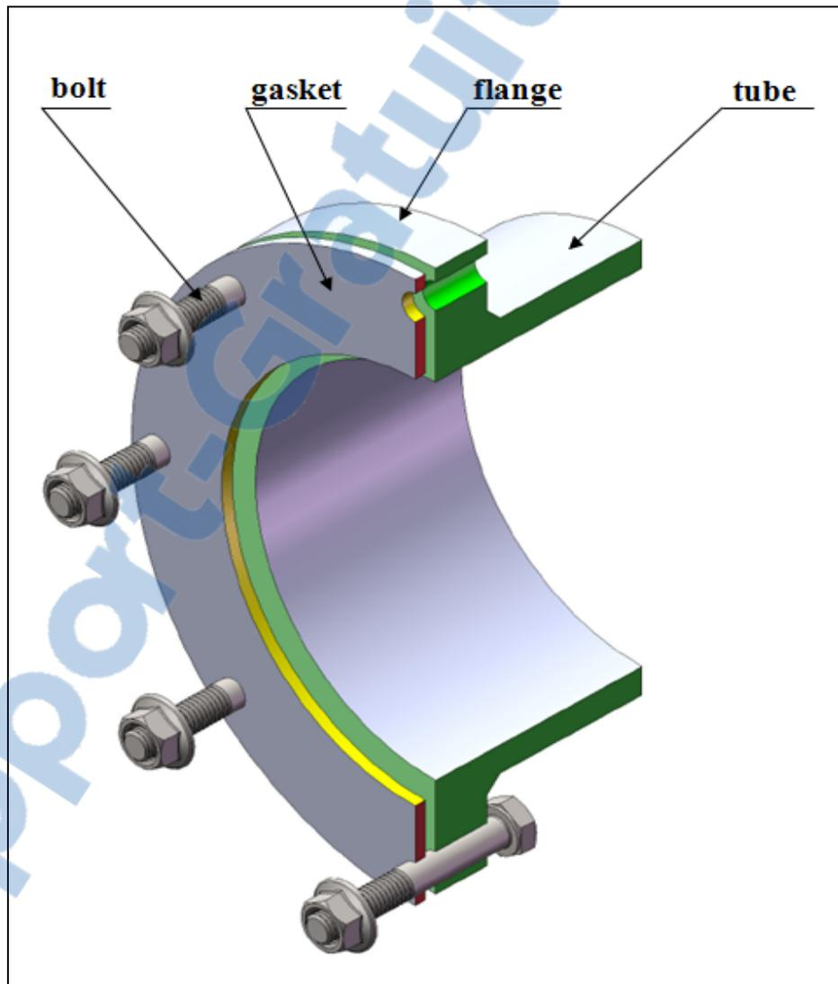
Figure 1.3 Bolted flange joint – full face types
