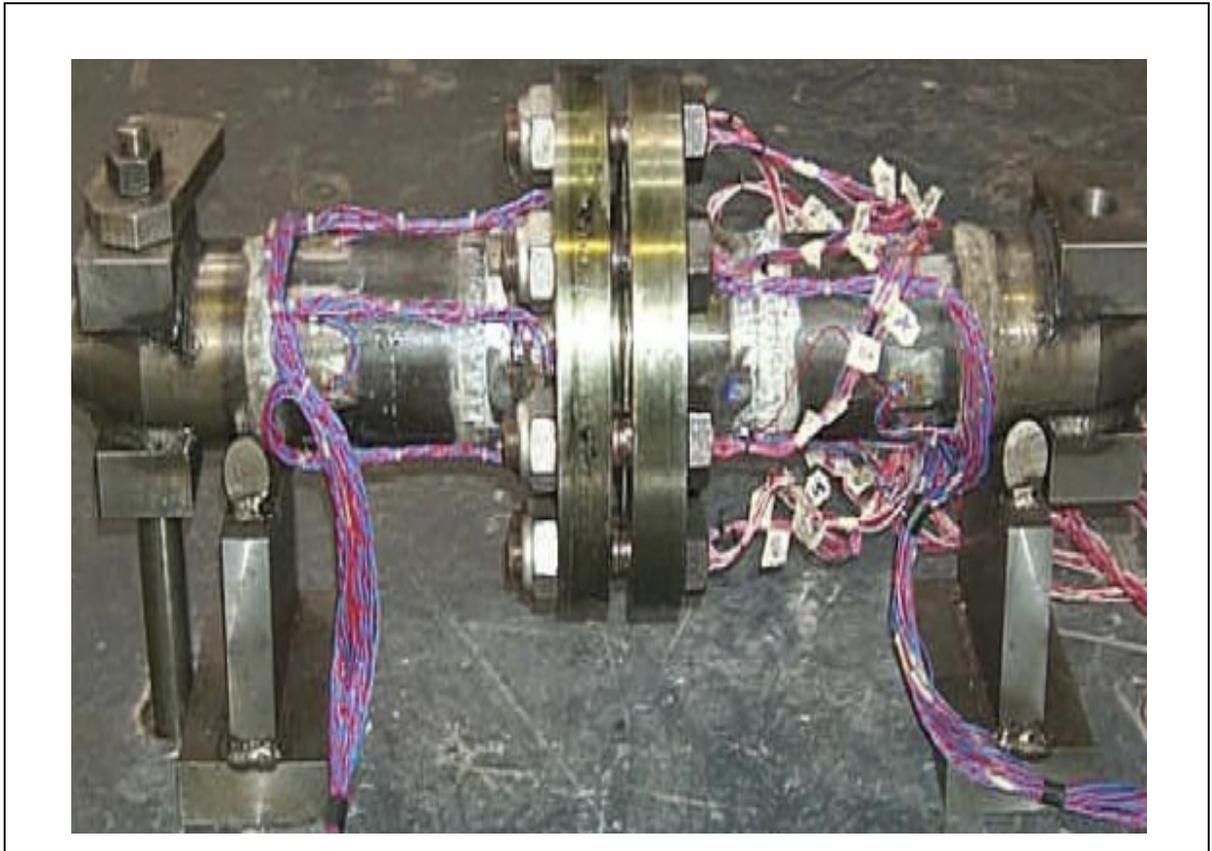
**Figure 2. 4 Experiment for bolted flange joints [13]**
