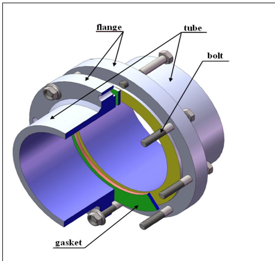
**Figure 1.2 Bolted flange joint – raised face type**
