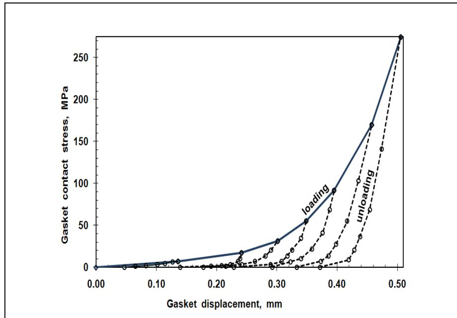
**Figure 1.5 Stress-strain relationship of CMS gasket [3]**
