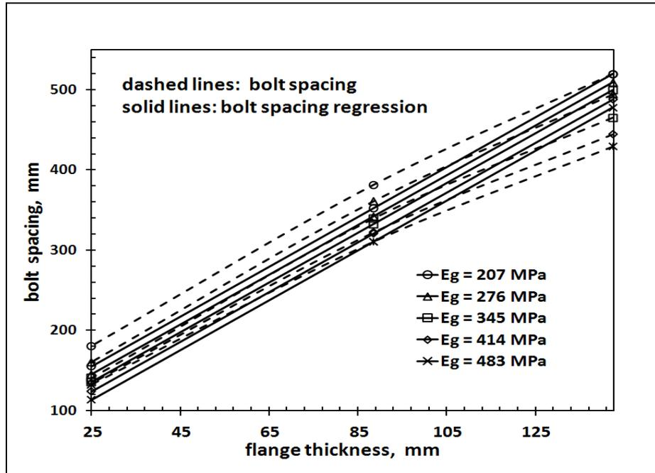
Figure 6.19 Relationship between bolt spacing regression and flange thickness; 52 in HE flange
