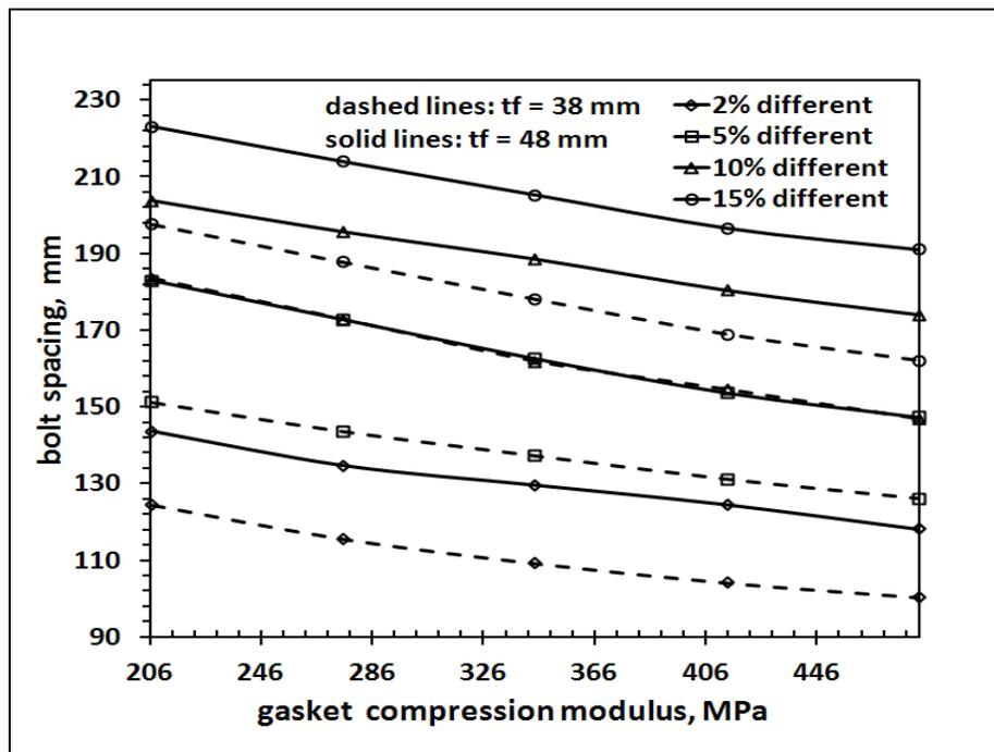
Figure 6.8 Relationship between bolt spacing and gasket compression modulus; 24 in. HE flange
