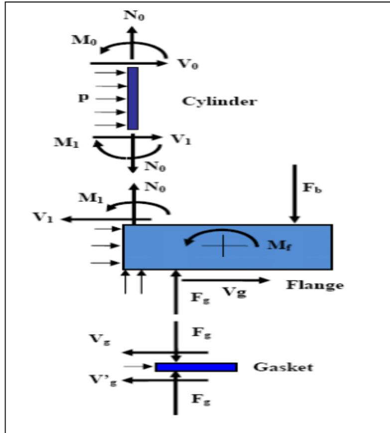
**Figure 3.1 Analytical model of bolted flange joint**
