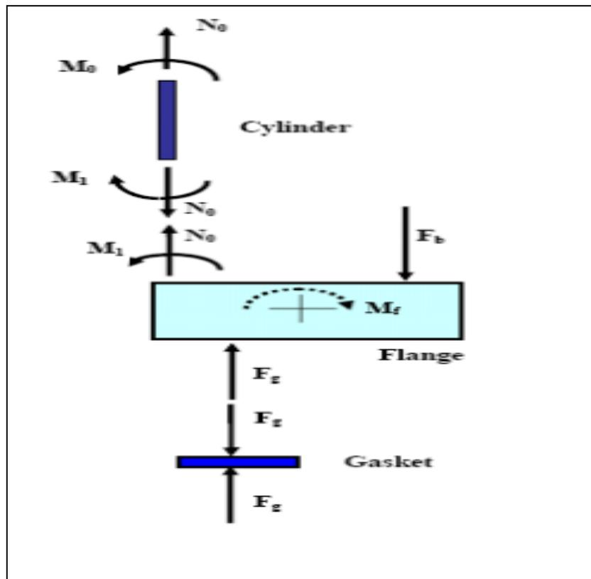
Figure 4.2 Loads in a bolted flange gasketed joint
