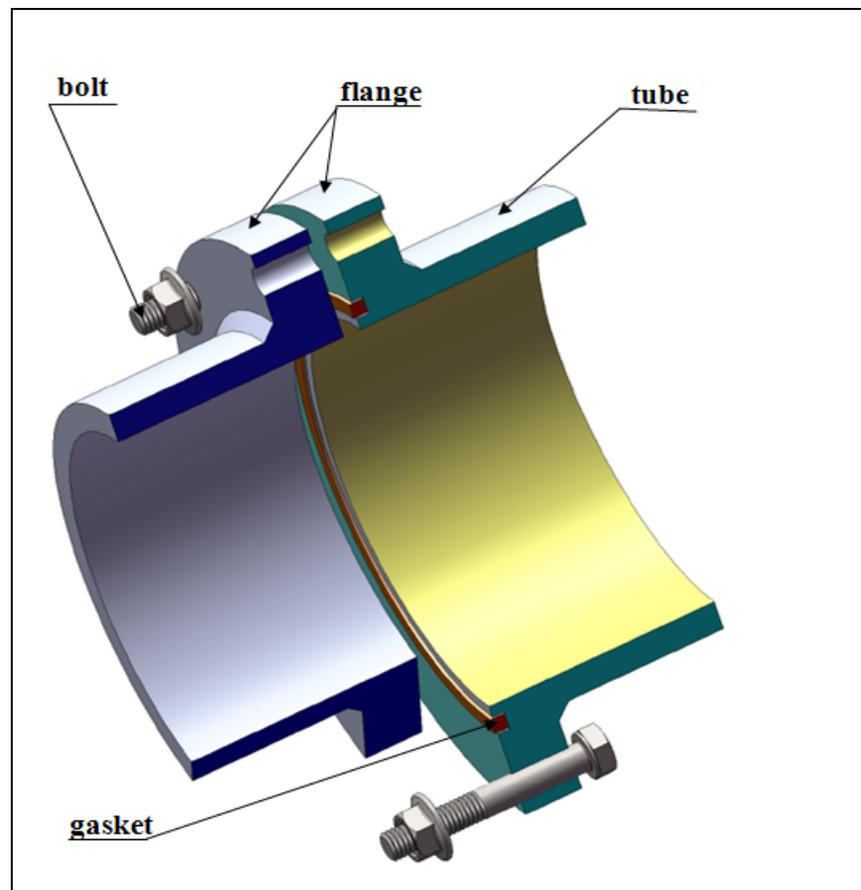
**Figure 1.4 Bolted flange joint – metal-to-metal contact type**
