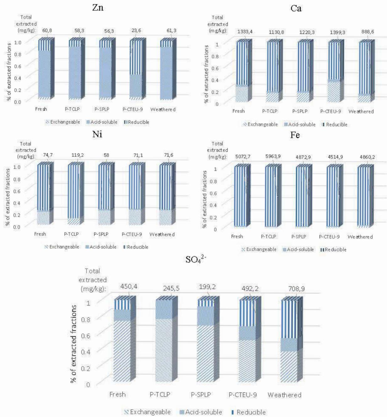
Figure 5-8 : Metals distribution after the leaching tests and the weathering cell tests for the mixture 2-H
