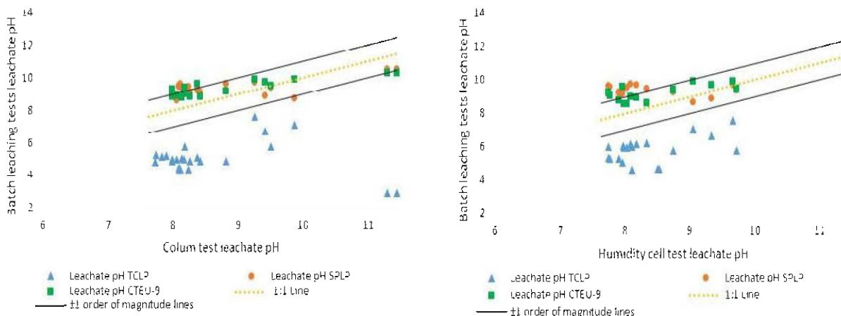
Figure 4-9 : Batch leaching tests pH compared to kinetic tests pH
