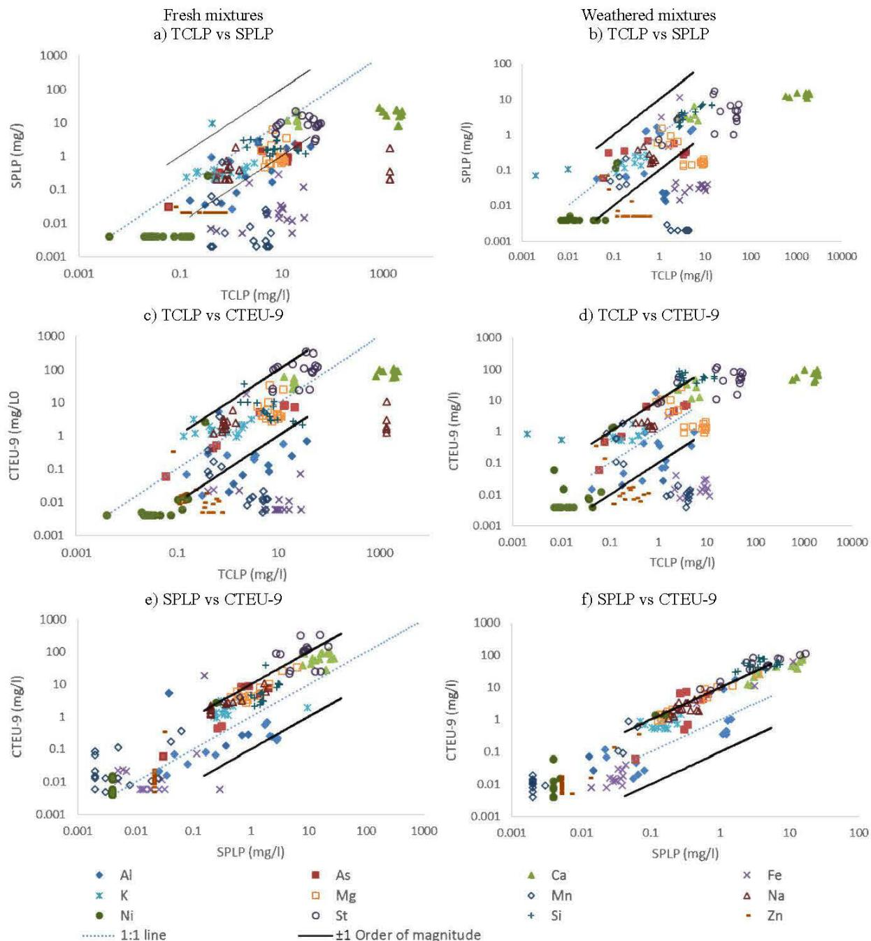
Figure 5-4 : Comparison of the leaching tests carried out on the fresh and weathered mixtures
