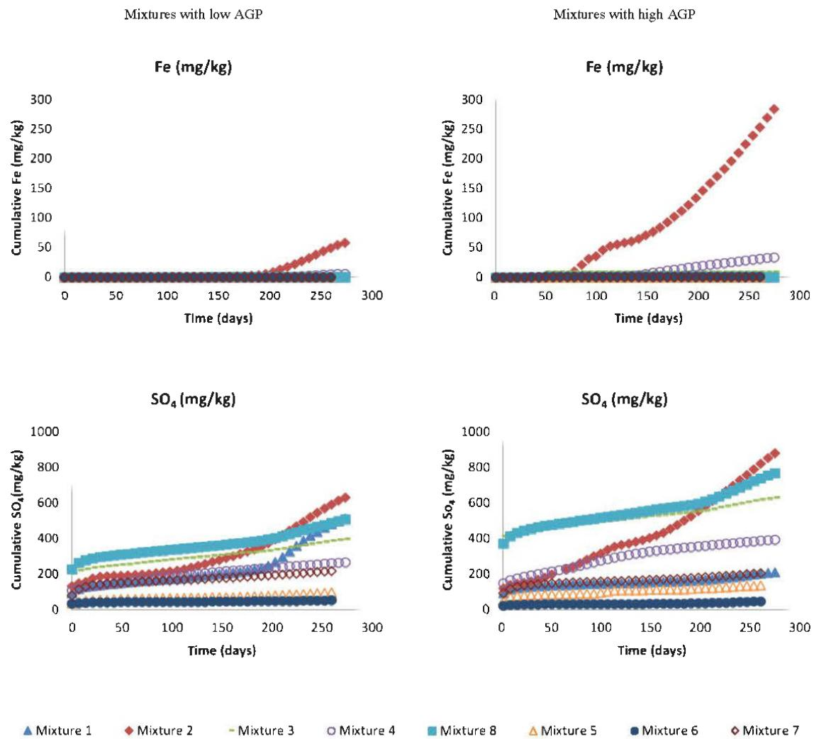
Figure 5-3 : Evolution of the total cumulative leached of Fe and SO<sub>4</sub><sup>2-</sup> during the weathering cell tests
