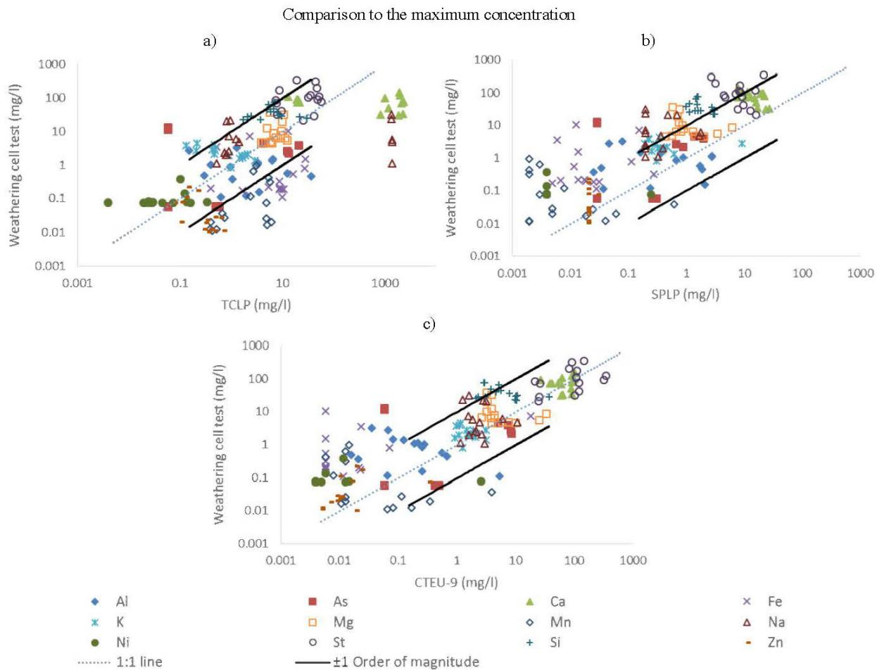
Figure 5-5 : Leaching tests results compared to the maximum concentration extracted by the weathering cell test
