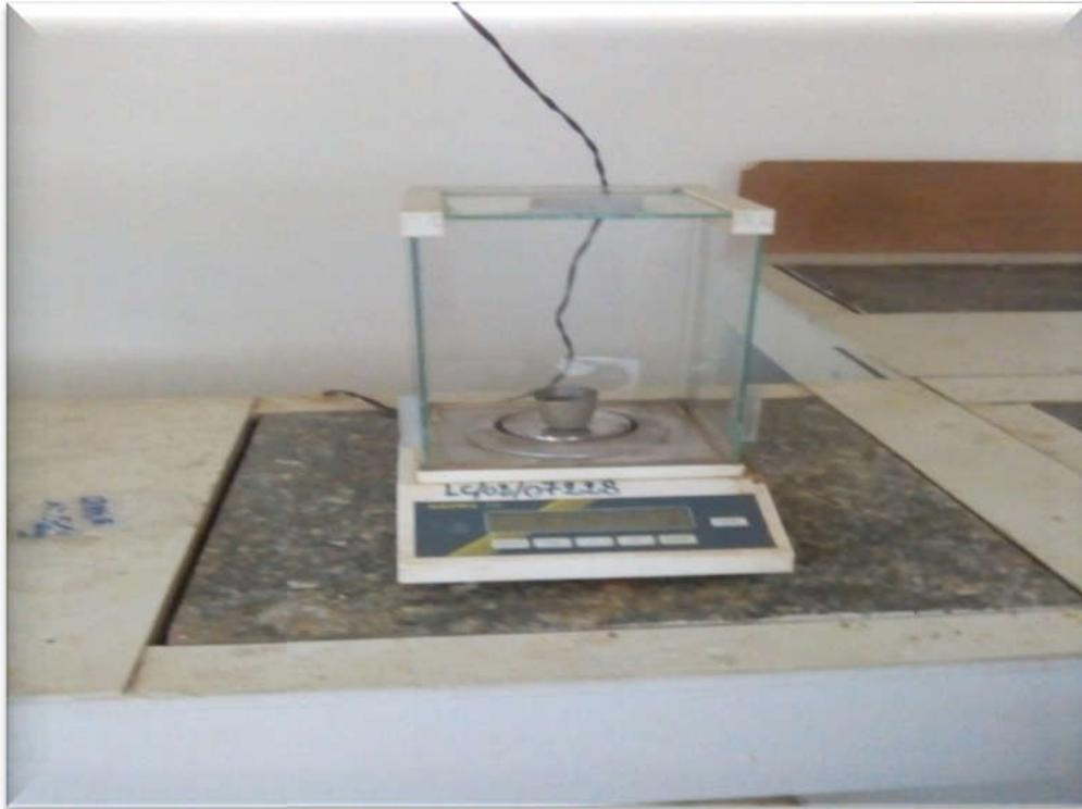
**Figure IV.34:** Balance analytique type KERN 770
