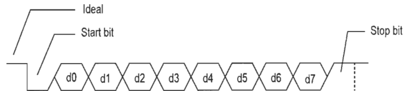
Figure 4-3 UART serial bit structure
