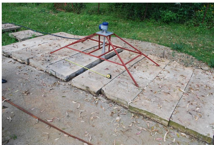
Figure 1 : sensor connected on the evacuation chamber, allowing to measure biogas outlet.
