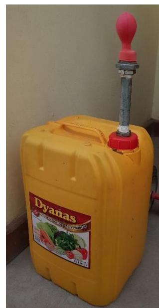
Figure 1: 20-liters jerrycan containing about 13 L slurry. The slurry is fed with about 1 L feed (cow dung, water, 1:1).
