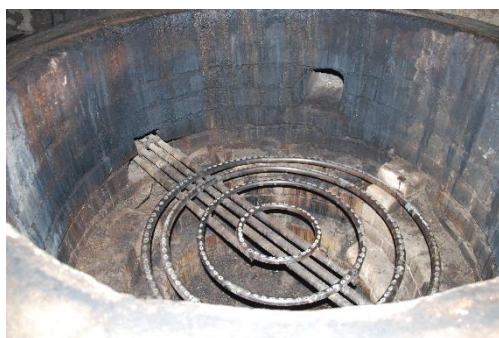
Figure 5: empty 400 L cooker with biogas burner.
