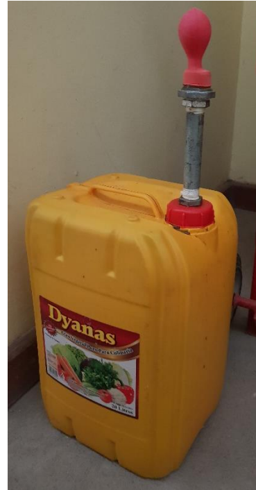
Figure 2: digester used for the digestion control. Note that plastic jerrycan should be avoided.
