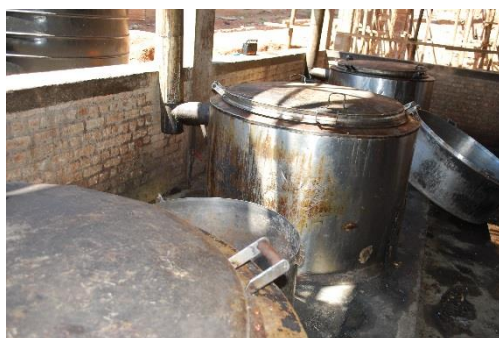
Figure 5: 400 L marmite, used for cooking with biomass (wood or biogas) in the prison.
