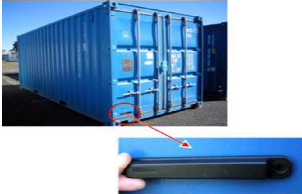
Figure 4.2 RFID tag attached on container (Leghorn seals, 2012).
