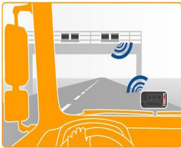
Figure 4.6 Wave recording sensor and DSRC Transponder (Info myto, 2012).
