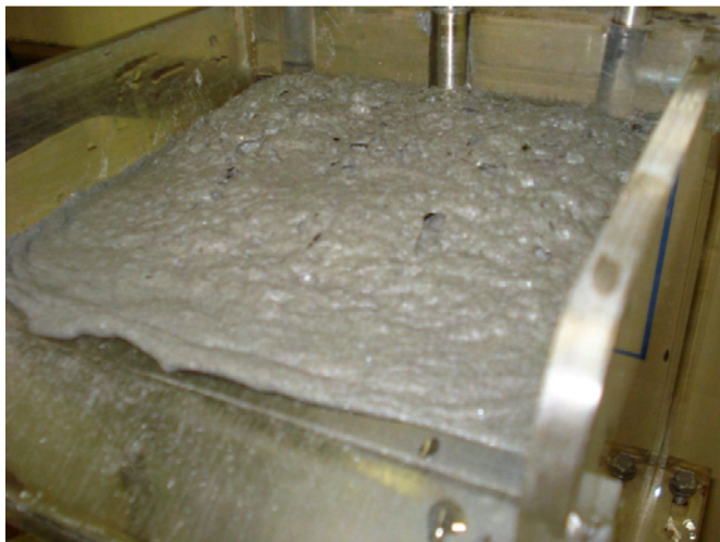
Figure A2.8: NHR froth for the -75+38 \mu\text{m} size fraction. Low froth height is obvious compared to Figure A2.2
