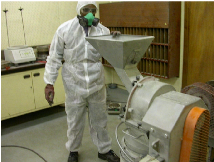
Figure A1.3: Picture showing full PPE gear employed during hammer mill comminution of PCB. The gear includes: N95 respirator, eye shield, laboratory coat and trousers, disposable hooded outer overall, safety shoe and ankle length PVC gloves with fabric inner lining.
