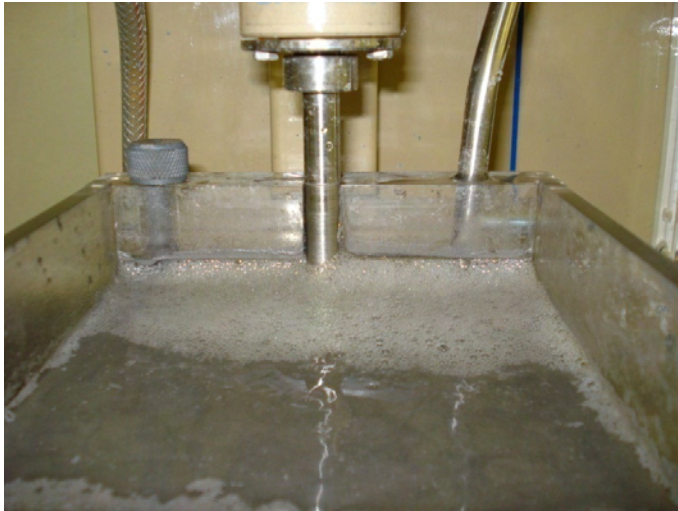
Figure A2.4: E21C at 28 min of flotation showing clean white unloaded froth A 59 seconds movie clip showing this froth bursting readily as they are not longer loaded is here .
