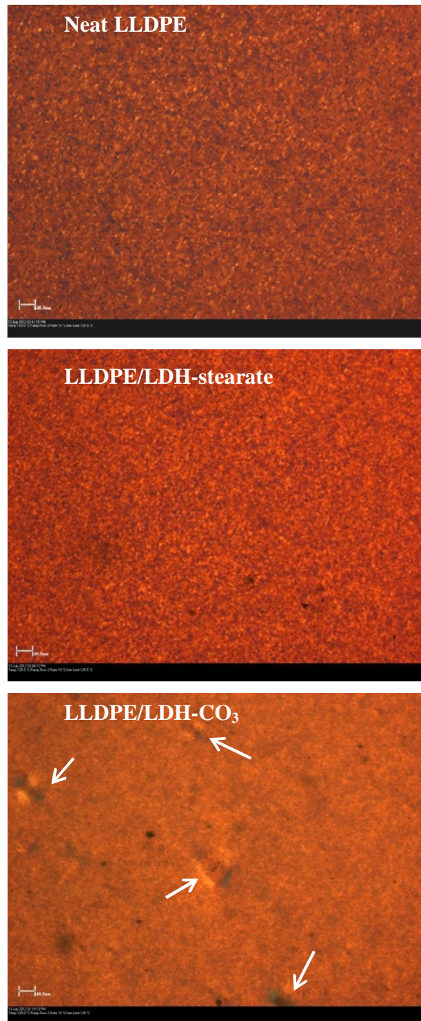
Figure 3.23. POM images of neat LLDPE and derivative composites (scale bar is 40 \mu\text{m} )
