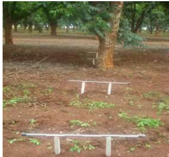
Figure 5.2 Hourly measurements of global solar radiation penetration through the canopy using Delta-T tube solarimeters positioned at various distances from the 37-year-old pecan tree row (0 m, 2 m and 4.5 m NNE – SSW) at the Cullinan experimental site, between 19 February and 02 March 2012.
