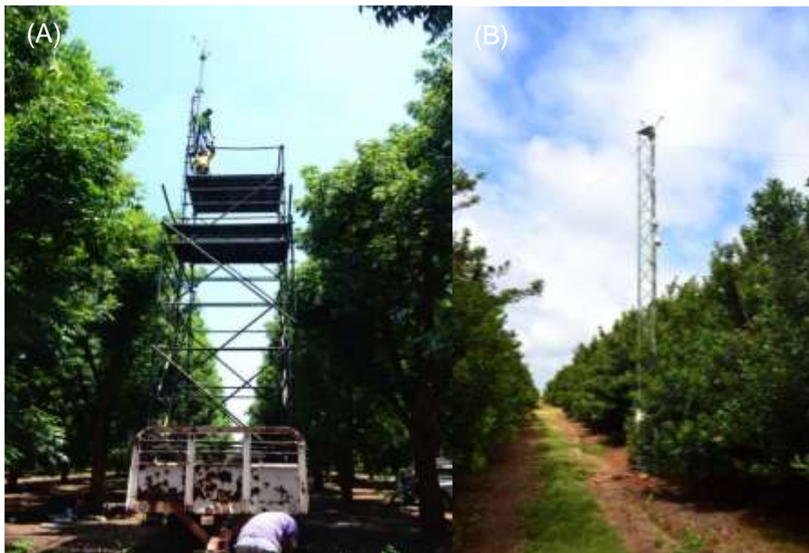
Figure 3.11 Position of the Open Path Eddy Covariance system on (A) scaffolding in the centre of the pecan orchard and (B) a lattice mast in the macadamia orchard.
