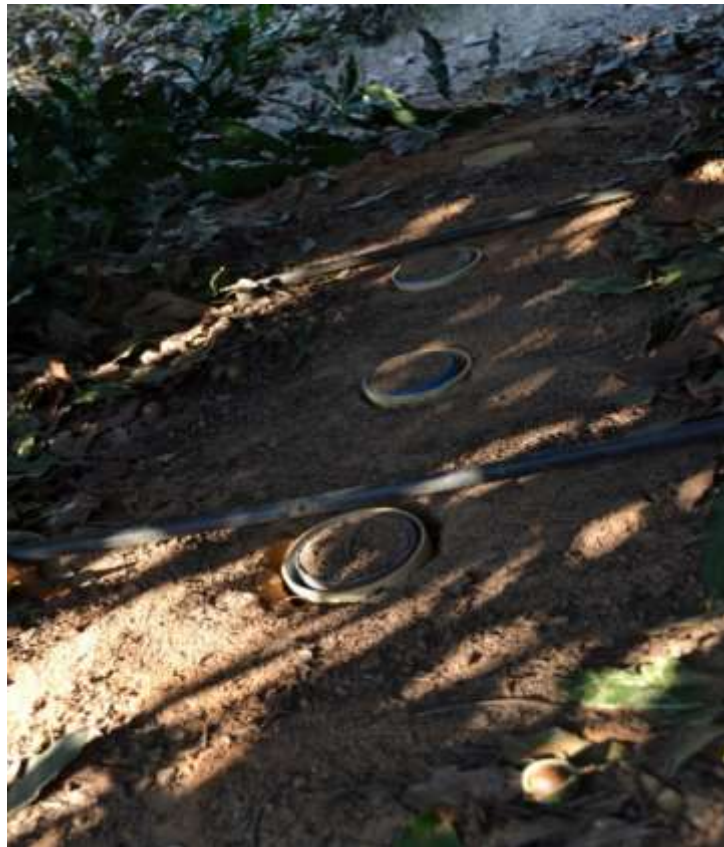
Figure 3.14 Micro-lysimeters used for soil evaporation measurements in 'Beaumont' macadamia orchard at White River experimental site.
