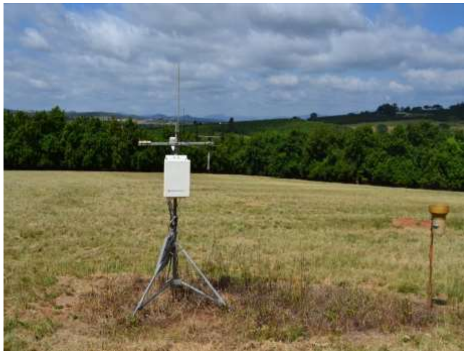
Figure 3.5 Automatic weather station installed in the macadamia orchard at White River experimental site.
