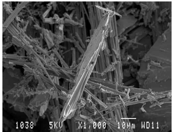
SEM images of calcium gluconate monohydrate recrystallised from water through diffusion with ethanol
