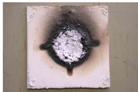
With AP750 coating: Left top – 60 sec exposure Right top – 180 sec exposure Left and right bottom – 960 sec exposure
