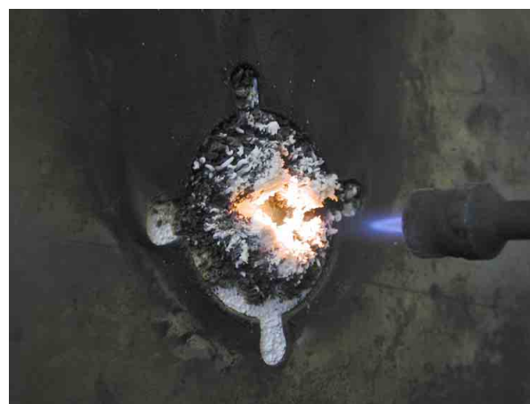
Gluconate/graphite/silica coating: Left – 600 sec, Right – 1800 sec
