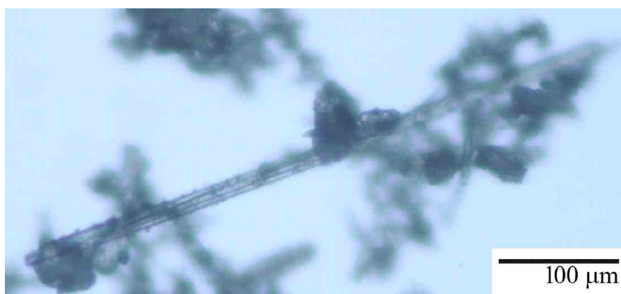
Figure 4-34 Light microscope images of commercial calcium gluconate monohydrate crystals (powder)
