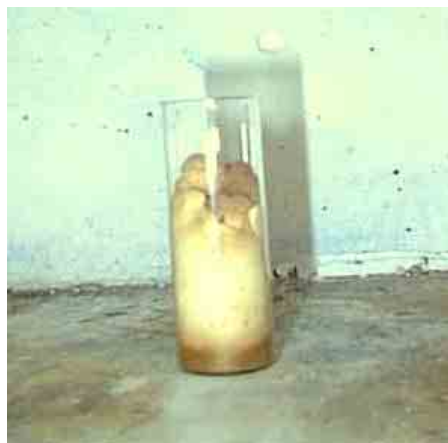
Figure 4-12 The calcium gluconate sample being foamed in the furnace at 300°C
