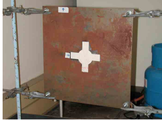
Rear view of the setup (no thermocouples)
