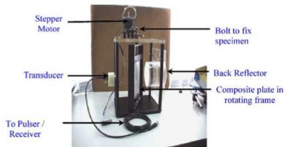
Fig. 4. Setup for back-reflection immersion technique.
