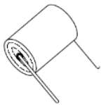
Wound capacitor, radial leads
