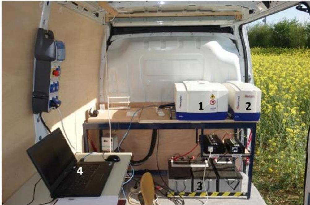
**Fig. 1** Mobile NMR laboratory with the NMR spectrometer including the magnet system and the probe assembly (1), the electronic control NMR unit (2), the battery (3) and a standard laptop computer for measurement control (4)
