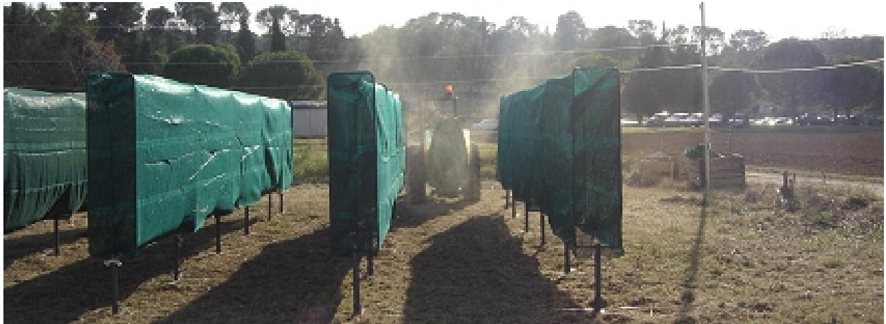
FIG. 4.10 – Experimental estimation of spray losses with an air-assisted sprayer.
