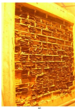
Fig. 11. Spalling-induced failure of load-bearing walls: (left) emerging parasitic bending moment induced by the eccentricity of vertical loading due to spalling, (right) scheme of the failure mode at the final stage of the fire test.
