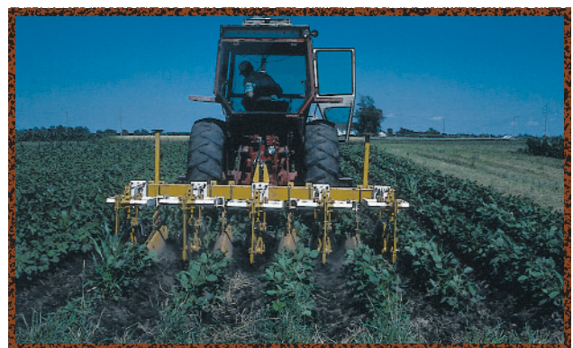
Row cultivators are used two to three times to control weeds between rows.
