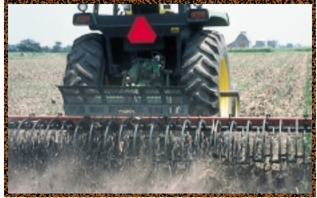
Rotary hoes or harrows are the first tillage operation used on organic farms.
