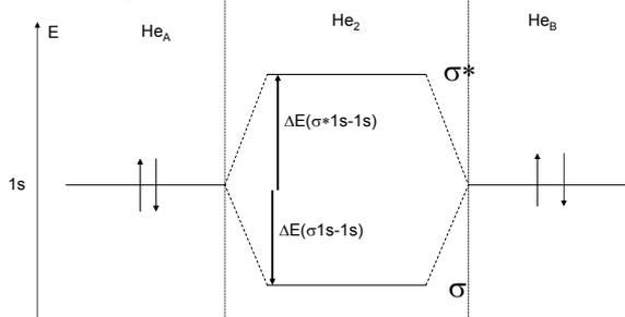
$$\Delta E = 2 \cdot \Delta E(\sigma 1s-1s) + 2 \cdot \Delta E(\sigma^* 1s-1s) > 0 : \text{ système moins stable}$$
