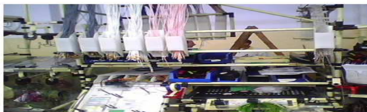
Figure 8: Cellule de kitting
