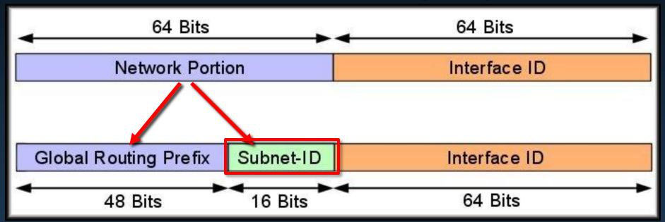
Using 16 bits for the Subnet-ID allows 65,536 separate subnets.....(that might be enough)...
