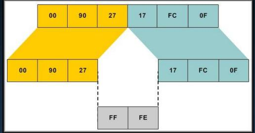
at the 24th bit of the MAC address to create a 64-bit, unique interface identifier.
