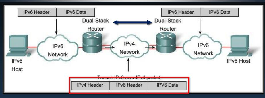
• When IPv4 is used to encapsulate the IPv6 packet:
