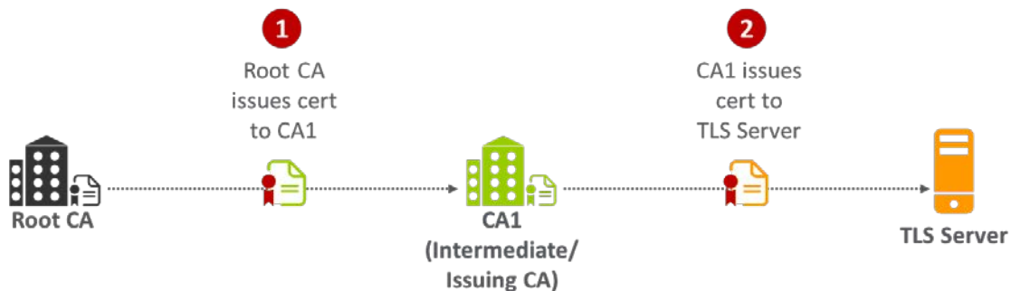
Figure 2-6 A Root CA Issues a Certificate to an Intermediate/Issuing CA, Which Issues TLS Server Certificates
