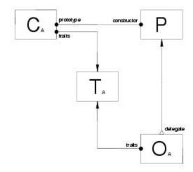
The value is a class object that has the form shown in the drawing above. The class object is CA. When used as a type, it evaluates to its instance traits (TA). When used in a new expression, the class serves as a factory object with a special method that creates a new instance (OA), which contains an internal delegate property pointing to the class object's prototype (P) and an internal traits property pointing to the class object's instance traits (TA).
