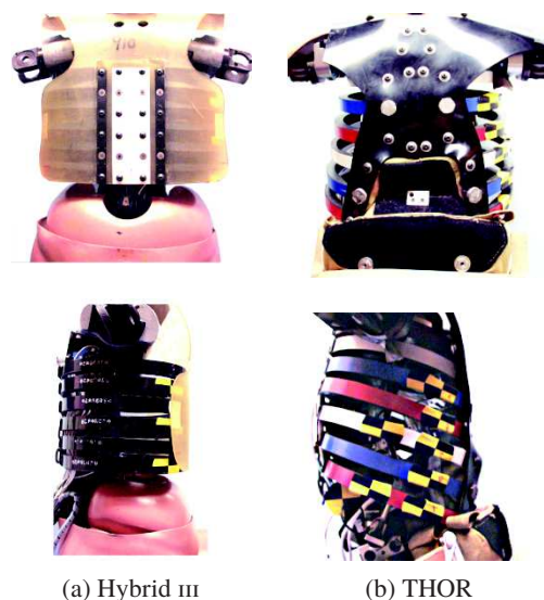
Figure 1.24 – Anatomy comparison between Hybrid III and the THOR dummy (Shaw et al. 2004)
