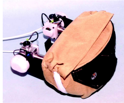
(e) THOR abdomen assembly view (THOR NT Manual, NHTSA/GESAC, Inc. 2005b)
