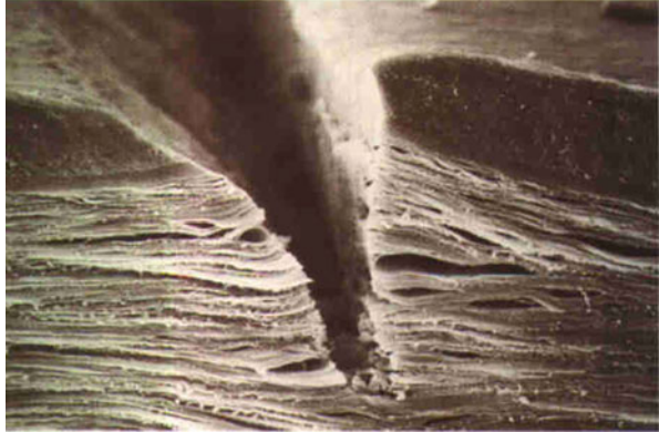
Fig. 2.2 Scanning electron microscopy of ablated cornea with a 211-nm laser (picosecond). Magnification 550x (Xin-Hua Hu, Ph.D., UC Irvine, CA, EEUU)
