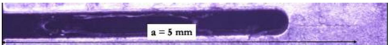
$N = 115.10^3$  cycles,  $\Delta K = 13,76 \text{ MPa.m}^{1/2}$  et  $da/dN = 1,33.10^{-8} \text{ m/cycle}$
