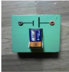
Figure 101: Support de pile 9 V
