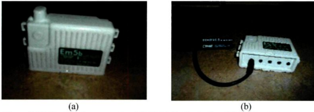
Figure 3.13 Devices for measuring LWC (a) Em5b device, (b) Ec-5 moisture sensor connected to Em5b device.
