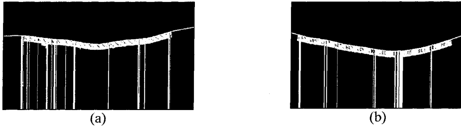
Figure 4.32 Snow shedding scenarios at (a) 42.9% shedding, (b)23.4% shedding. Conditions: Period 0.9072 s, Motor speed level-3 and LWC 15-18%, 18-20%.
