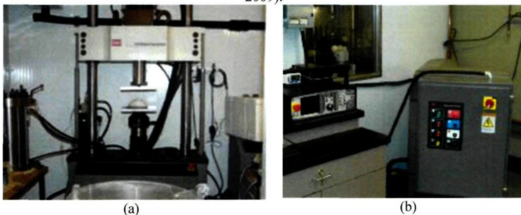
Figure 3.8: (a) Material testing machine (MTS), (b) Drivers for MTS machine.
