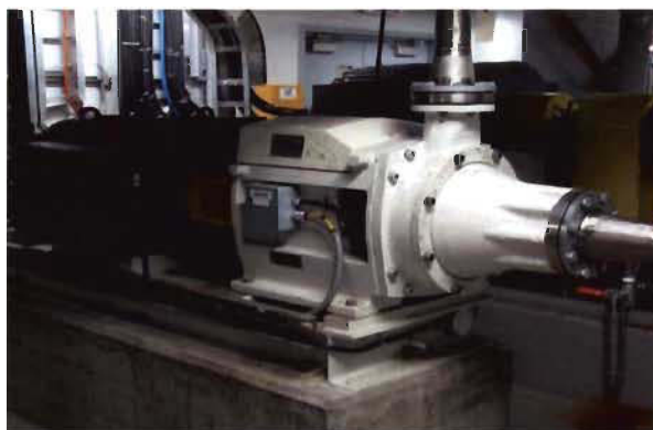
Figure 3.5 Raffineur conique Valmet RF-0
