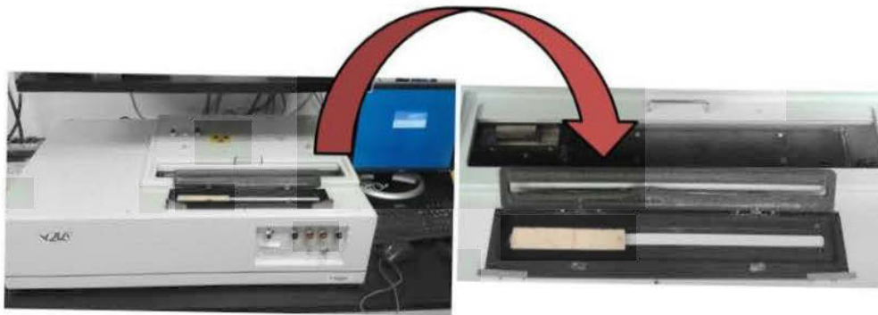
Figure 3.4 Densitomètre QTRS-01X Tree Analyser de Quintek Measurement System, Inc. (QMS) (Source : Quintek Measurement System, Inc. )
