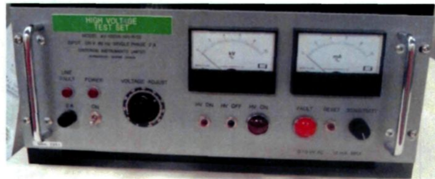
Figure 45 : Source haute tension 10 kV c.a.
